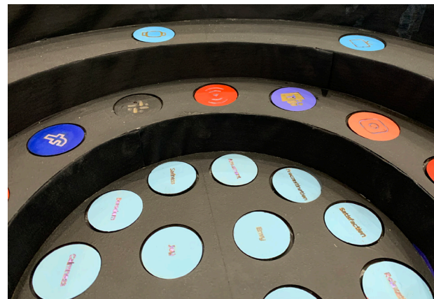
Figure 4.28 - Buttons with resin and LED lights
